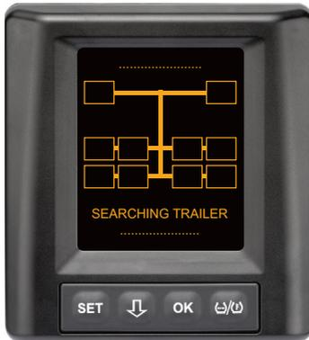
The CPC system is ready for operation. Tire data is displayed just after the journey begins. The automatic trailer detection (ATL) is not yet complete.
