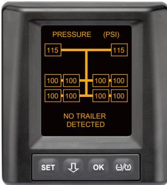
Data is received for all truck wheel positions, the automatic trailer detection (ATL) is not yet complete however, no trailer with tire sensors was found.
