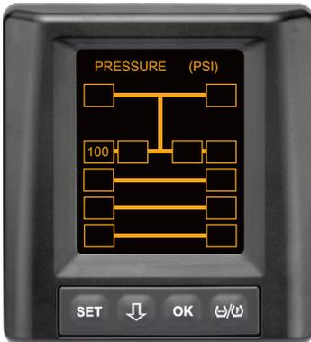
Tire data is received for the wheel position of the 2nd outer left axis.
