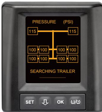
Data is received for all truck wheel positions and the automatic trailer detection (ATL) is not yet complete.
