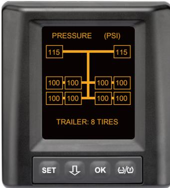
This display appears when the conditions for automatic trailer detection with tire position are not met and the values for inflation pressure and temperatures inside the tire are within the permissible value range.
