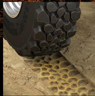
**Special tread design with multiple block geometries**
